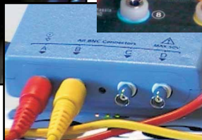
CTB Probe Lead (BNC) Scope Connection
