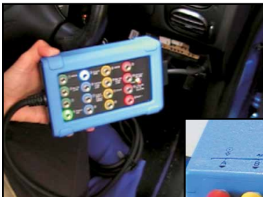
CTB Connected to Vehicle DLC
