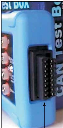
CTB 16 Pin Pass-Thru Connector
